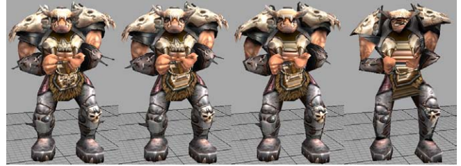
TGE Orc drawn at various levels of detail: LOD #0 with 2430 polys (far left), LOD #2 with 2203 polys, LOD #4 with 1259 polys, and LOD #6 with 353 polys.
